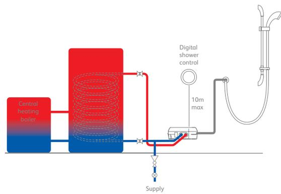
Typical combination boiler installation
