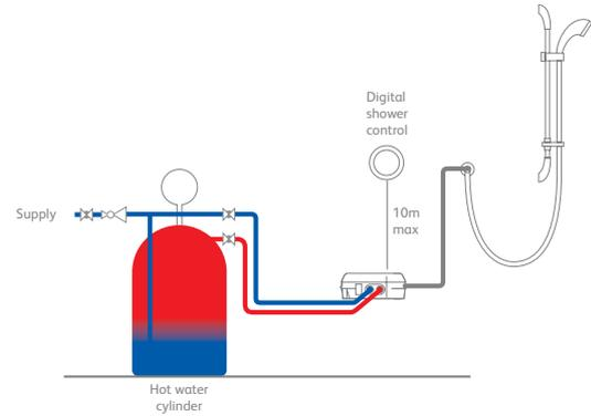
Typical pumped system installation
