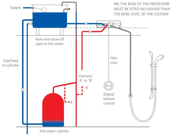
Typical Thermal storage unit system installation
