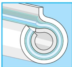
It is made up of 5 layers, the centre of which is a blue coloured oxygen barrier which prevents the ingress of air into the system, thereby reducing the effect of corrosion on metal components.
