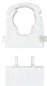
The second type uses a screw and therefore takes a little longer to fix. When pipes are required to cross over, it is possible to add a spacer to the clip. This will give room between the pipe and the wall to allow the pipes to cross over. If pipework needs to be insulated, using the spacer will give room for the lagging to be applied.
