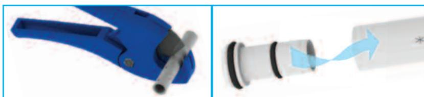
Ensure the pipe is free of score marks. Cut the pipe square. When using Speedfit Barrier Pipe cut along an insertion mark. We recommend the use of JG Pipe Cutters.
