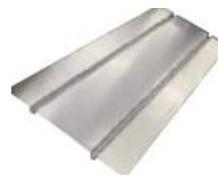
Spreader plates are available for timber flooring using either traditional joists or TJI joists. The plates absorb the heat from the pipework and spread it evenly across the floor decking above.
