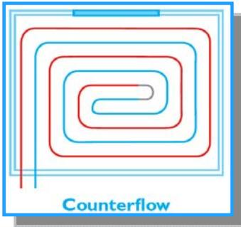
Counterflow is a common circuit pattern to use, it can sometimes be referred to as a spiral pattern. This pattern achieves an even floor temperature with alternating flow and returns.
