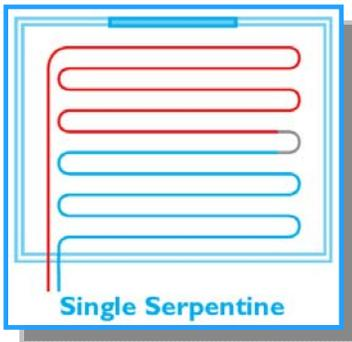
Serpentine is a simple up & down circuit pattern. It is especially good to use when you have irregular shaped rooms or small areas such as kitchens and utility rooms. This pattern is also used for the Spreader plates systems.
