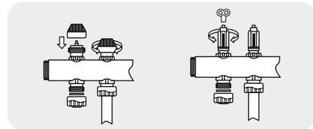
Once all of the circuit flow rates have been adjusted, the system should be left to operate for a short period whilst any remaining air is removed.
