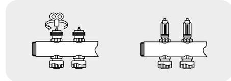
When adjusting the manifold flow rates, care should be taken to ensure that the adjustment spindle is not left with any of the thread showing.
