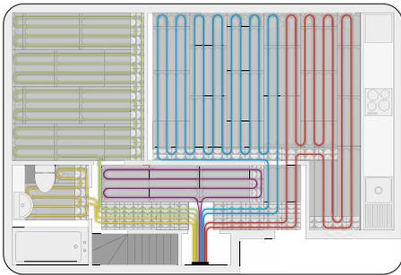
In transition areas such as hallways and corridors a combination of end return/transition and full panels can be used in order to accommodate the pipe connection lengths and any dedicated circuit(s) for that area.
