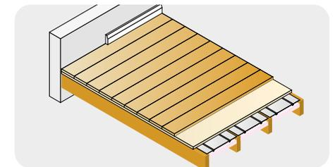
If a manufactured timber floor is to be used then it is recommended that this be of a suitable load bearing quality. (Please request advice from the specialist flooring supplier.)
