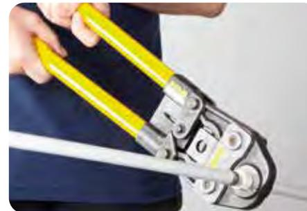
Extension pieces are included with the Eco Press if extra leverage is required to completely close the tool. Only when the tool has been completely closed with the two stops touching is the fitting fully secured. The levers can then be opened and the fitting will be released from the jaws.
