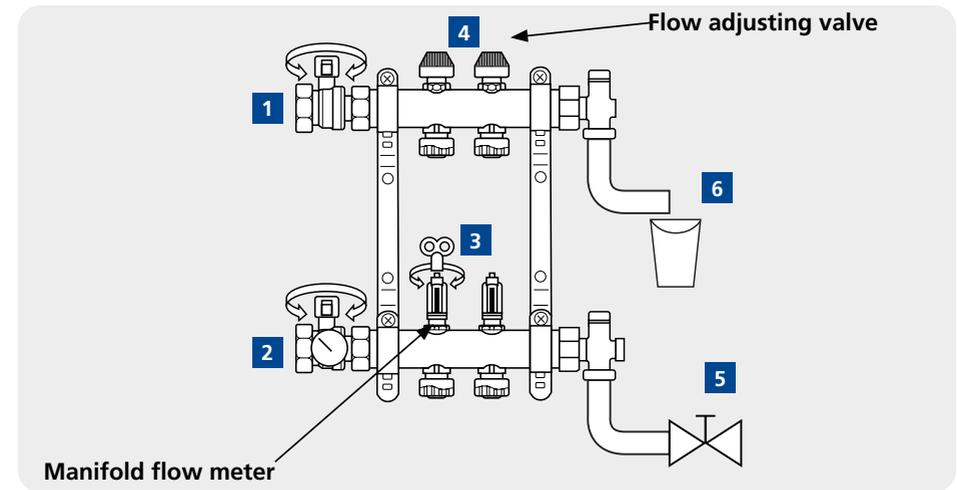
First, close the manifold isolating valves (1) and (2). Then connect a hose pipe to the manifold return drain off point (6) and take to a drain. Connect a second hose pipe to the manifold filling point (5) and attach to mains cold water supply (3 bar max). The connections to the manifold drain and fill points are ¾" BSP. Use flexible ¾" tap connectors for the simplest method of connection.
