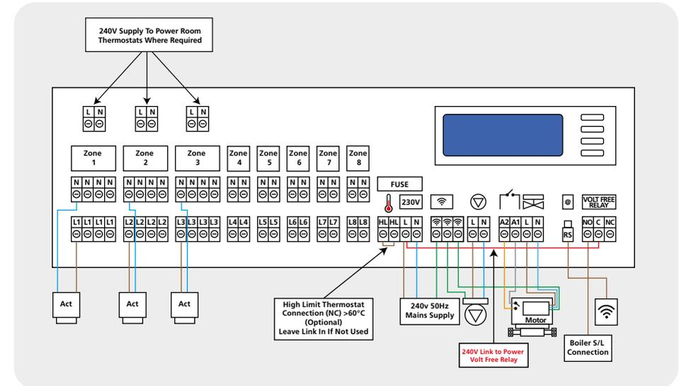
If fitting without a Zone Valve, ensure that the factory fitted link across terminals A1 and A2 is in place.
