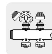
Remove the blue cap from the manifold return port and, using the bleed key provided, turn the flow adjustment spindle clockwise to completely close the circuit.
