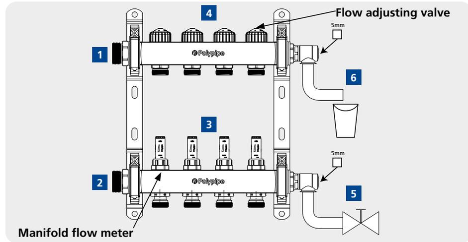
First, close the isolation valves (1&2) to the system. Then connect hose pipes to the manifold drain/ fill points.
