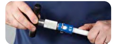
The chamfer tool should be twisted gently to provide a lead in. Any debris should be removed from the pipe end and the chamfer tool. Check that the pipe has been cleanly chamfered around the full diameter of the pipe.
